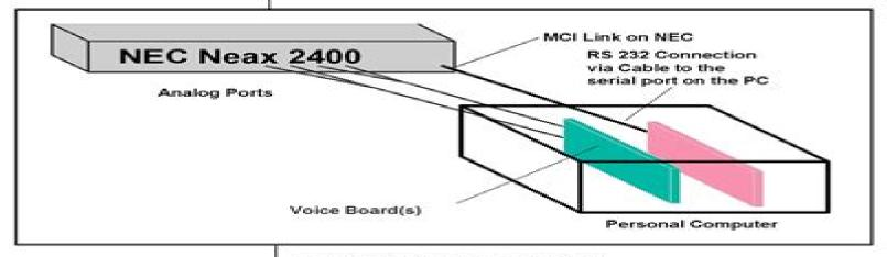
Communications between the Neax 2400 and the Smooth Operator are through a RS-232 Connection to the serial port on the PC.
