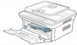
3. Thoroughly roll the cartridge five or six times to distribute the toner evenly inside the cartridge.
