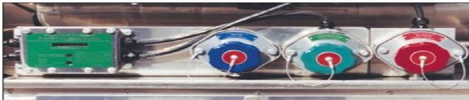
Scully truck mounted control monitor and sockets
