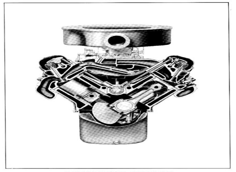
Fig. 6-2 Transverse Cross Section of Engine (Front View)
