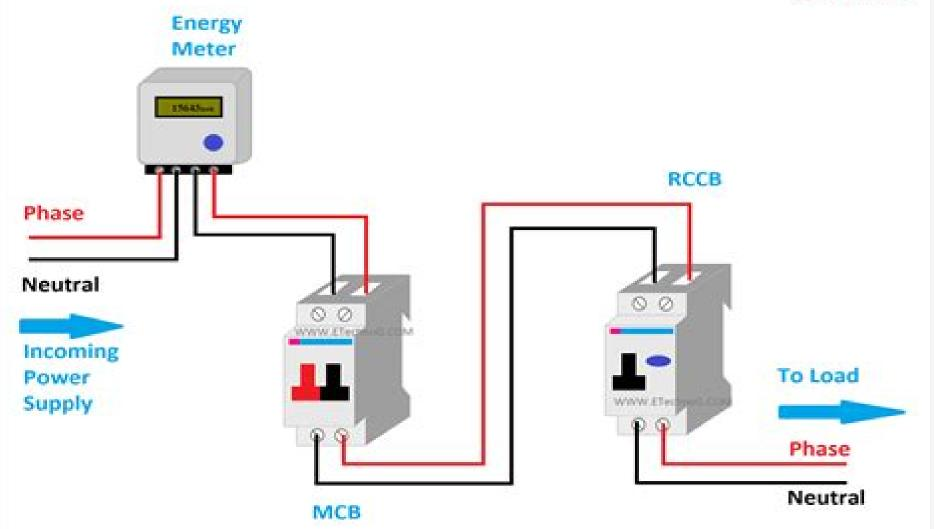
RCCB Connection Diagram with MCB
