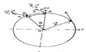
A motion in which a farticle moves along the circumference of a circle or traces an angle is said to be a circular motion.
