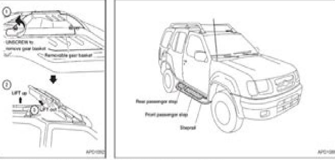
The roof rack is equipped with a removable gear basket. The maximum gear basket load is 30 to (13.6 kg) evenly distributed. The gear basket can be removed by unscrewing the four hold down botts.
