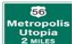
INTERCHANGE ADVANCE EXIT SIGN
