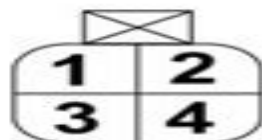
CRANK ANGLE SENSOR CONNECTOR ON ENGINE WIRING HARNESS
