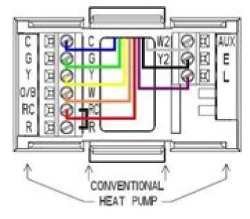
Select the correct letter designations to follow for your system. If you have a standard heating and/or cooling system, use the CONVENTIONAL letter designations. If you have a heat pump system, use the HEAT PUMP letter designations to wire the new thermostat.
