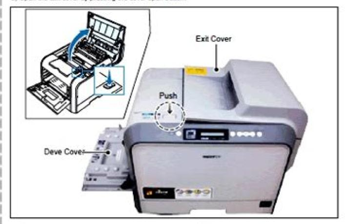
Caution: Before opening the exit over completely open the DEVE cover until it is at right angles to the main frame and the toner cartridges are ejected
