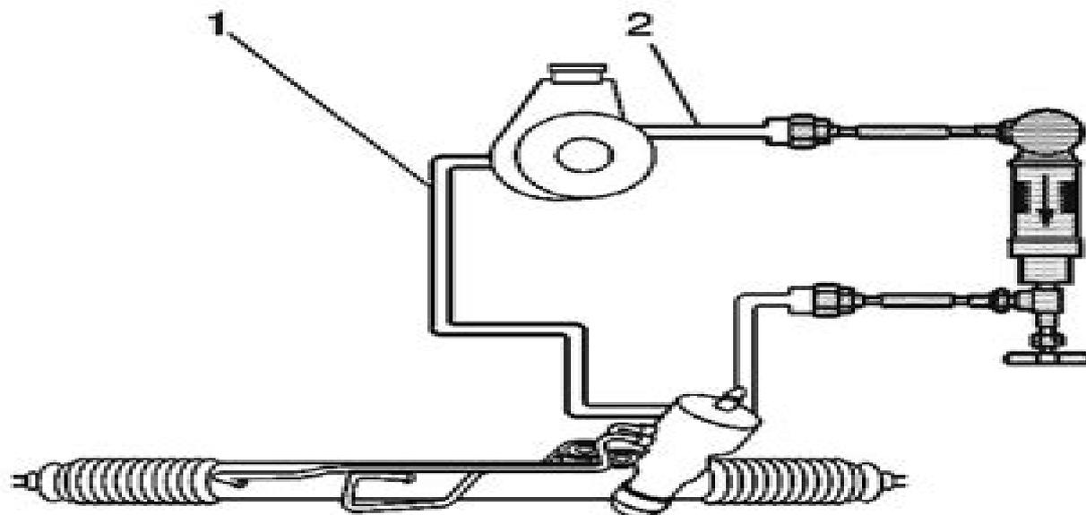
**Fig. 3: Testing Rack and Pinion System Pressures**
