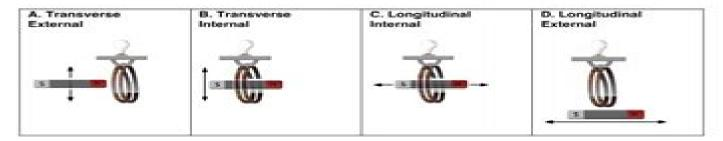
4. Move the bar magnet through the coil and observe the motion of the electrons in the forward arc of the coil loops. Report the correlations of magnet motion and electron motion.
