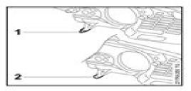
Sprocket cover with integrally moulded chain catcher (1).
