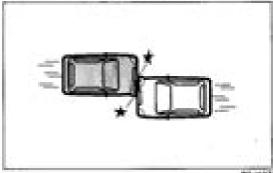
Collision angle is offset from the vehicle angle (offset collision)
