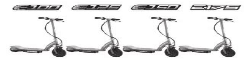
A NOTE: The E100/E125/E150/E175 must be traveling up to 3mph before motor will engage. Kick start up to 3mph while applying the throttle to engage motor.
