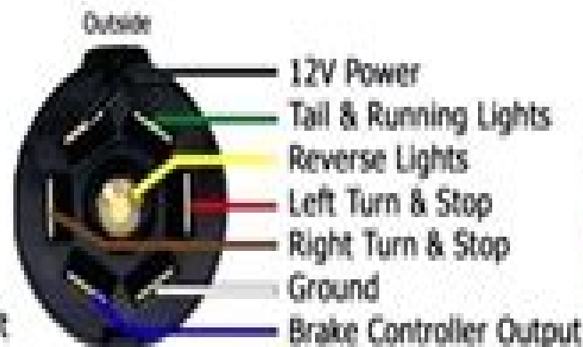
7-Way RV Standard (5th Wheel/Travel Trailer/Camper)
