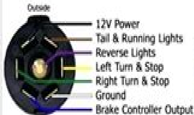
7-Way Traditional (Utility/Equipment/Cargo Trailers)
