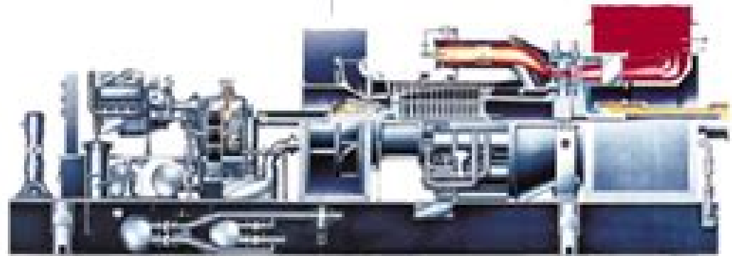
MS5001 Gas Turbine
