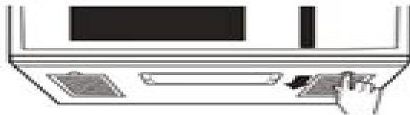
2. Soak the grease filter in hot water and a mild detergent. Rinse well and shake to dry. Brushing the filter lightly can remove embedded dirt.
