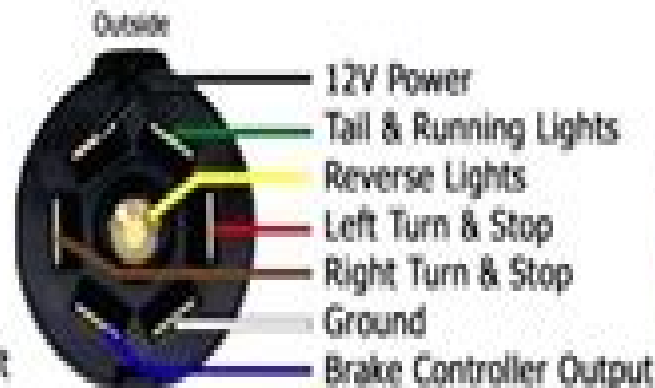
7-Way RV Standard (5th Wheel/Travel Trailer/Camper)
