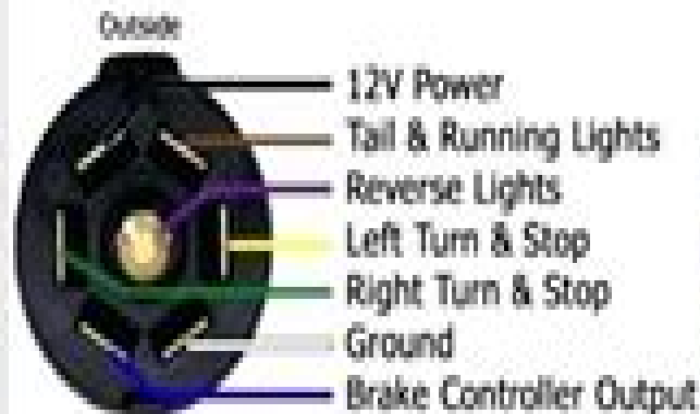
7-Way Traditional (Utility/Equipment/Cargo Trailers)
