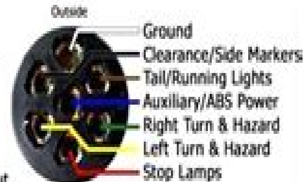
7-Way Heavy-Duty (Commercial/Agriculture Trailers)
