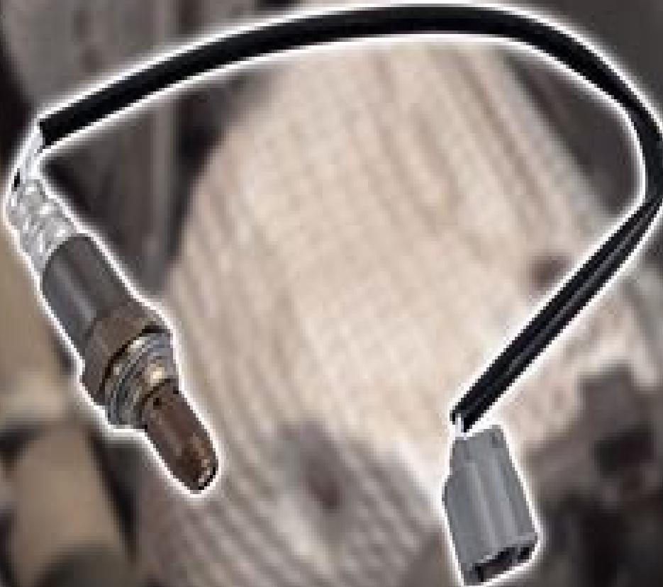
**HOW TO REPLACE UPSTREAM O<sub>2</sub> OXYGEN SENSOR
