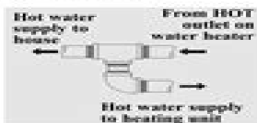
Tee fitting for horizontal hot water supply lines.
