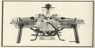
f you take two 65 cubic inch displacement single cylinder 4-stroke engines noted for their high level of performance and join them together with a common cramkcase and crankshaft, what do you have? You're right — a real strong running 1.3 cubic inch displacement 4-stroke twin. This is basically what Saito has done with their FA-130 twin, the subject of our engine review
