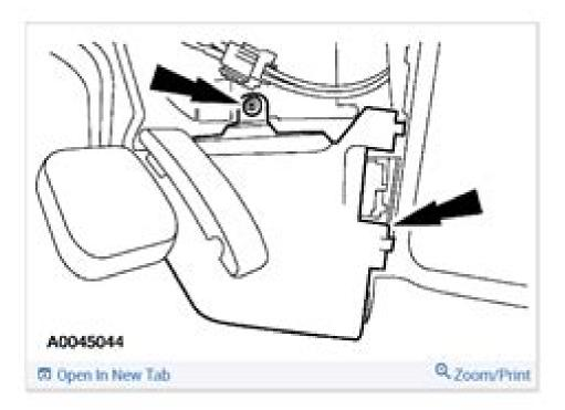
2. Remove the pin-type retainer and the lower shield.
