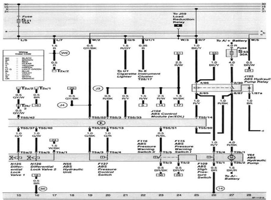
201 ABS with Electronic Differential Lock (EDL) Passat
