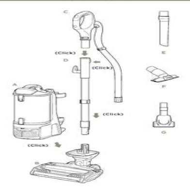
NOTE: For proper operation, ensure all parts are firmly CLICKED into place.
