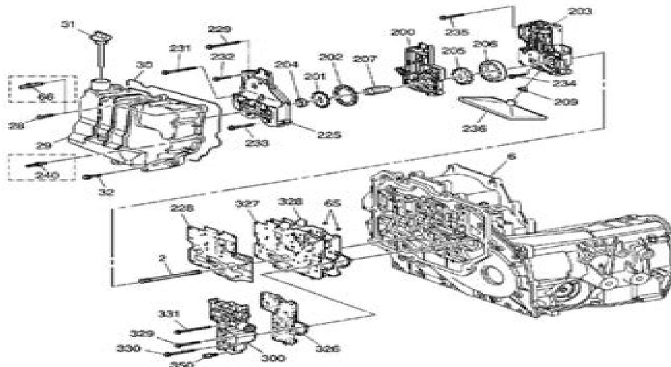
**Fig. 2: Transmission Case and Associated Parts Disassembled View (2 of 3)**
