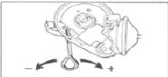
Fig. 8-9 "Cassette" type contact points adjustment
