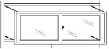
STEP 1. Center window in the opening. Make sure that the sash look is positioned to the INSIDE of the structure.
