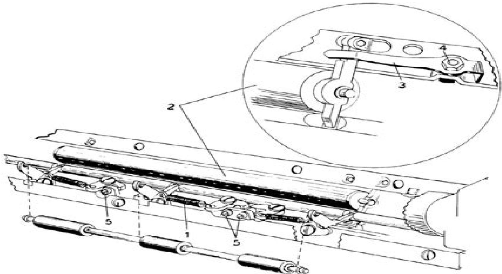
Proper paper feed depends almost entirely upon the condition of the platen and the feed rolls. If these are in good condition, your paper feed problems are about solved. Review the platen and feed roll pages of the General Information Section. This information will help you determine if a new platen or new feed rolls are necessary.
