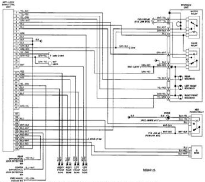
Fig. 20: Anti-Lock Brake System (ABS) Wiring Diagram
