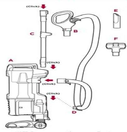
NOTE: For proper operation, ensure all parts are firmly CLICKED into place.
