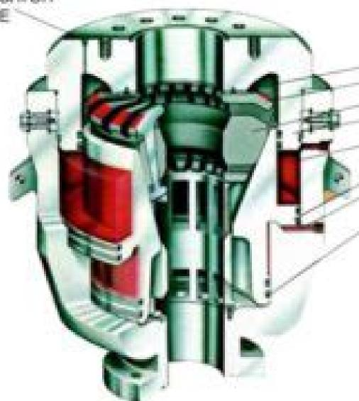
WEAR PLATE FLANGED STEEL INSERTS PACKING UNIT HEAD OPENING CHAMBER PISTON CLOSING CHAMBER SEALS
