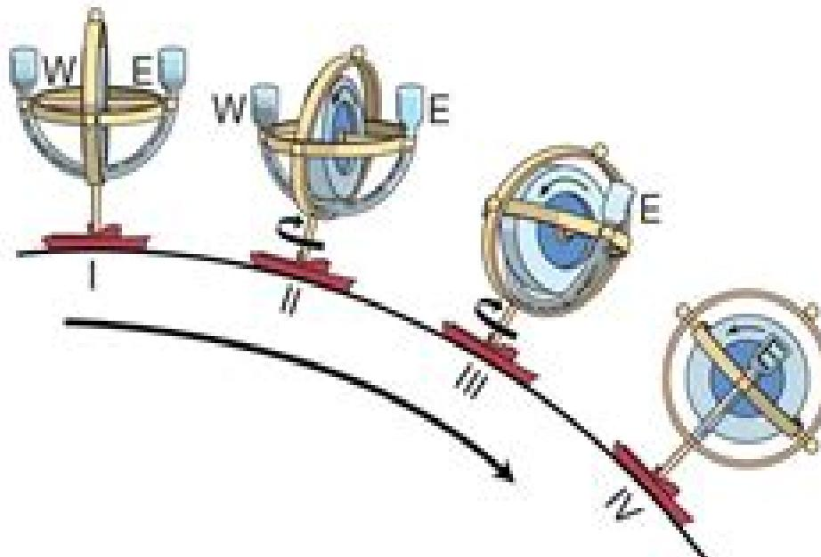
Rotation of Earth carries ship from west to east, regardless of ship's own movement, so that axis of gyroscope always becomes tipped from horizontal unless it is pointing due north and south.
