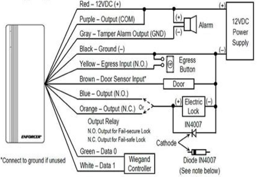
NOTE: For DC-powered electric strikes, connect the included diode as close as possible and in parallel with the electric strike. This absorbs possible electromagnetic interference to prevent operation of the strike from damaging the reader. Do not connect a diode when using electromagnetic locks or with AC powered strikes.
