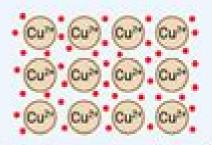
Copper ions immersed in an electron cloud
