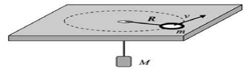
A disk of mass w is placed on a frictionless table, and attached to a vertically-hanging mass M by a string that passes through a frictionless opening in the surface. The disk has a speed v as it travels in a circle with a constant radius R. How much work is done on the disk in one half revolution?
