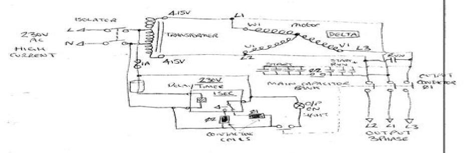
Ø2 = Single Pole contactor Ø1 = 4 Pole contactor
