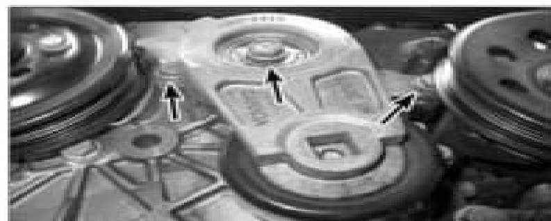
24.25 Typical V6 tensioner mounting fastener locations.
