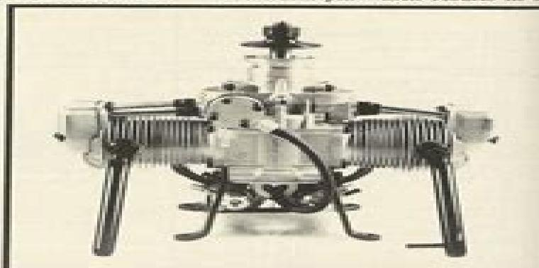
If you take two .65 cubic inch displacement single cylinder 4-stroke engines noted for their high level of performance and join them together with a common crankcase and crankshaft, what do you have? You're right—a real strong running 1.3 cubic inch displacement 4-stroke twin. This is basically what Saito has done with their FA-130 twin, the subject of our engine review
