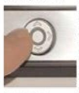
The 4-way control pad is used to select the active timer preset mode and to edit the timer values. The different types of mode available are: BLITZ, TOURNAMENT, GAME, and USER
