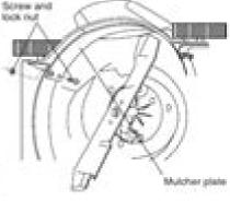
MULCHER PLUG BUILT INTO REAR DOOR
