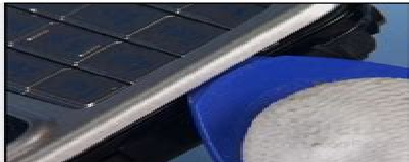
6. Unlock the plastic clips of the A-COVER with the SRT-6...
