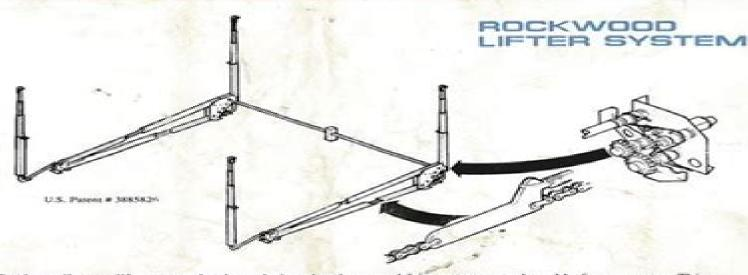
Rockwood's easy lifter as seem has been designed and patented for easy set up and trouble-free operation. This system is chain driven and cableless, is above the floor and eliminates the problem of breaking, streching, fraying and corrosion come on associated with cable lifter systems.
