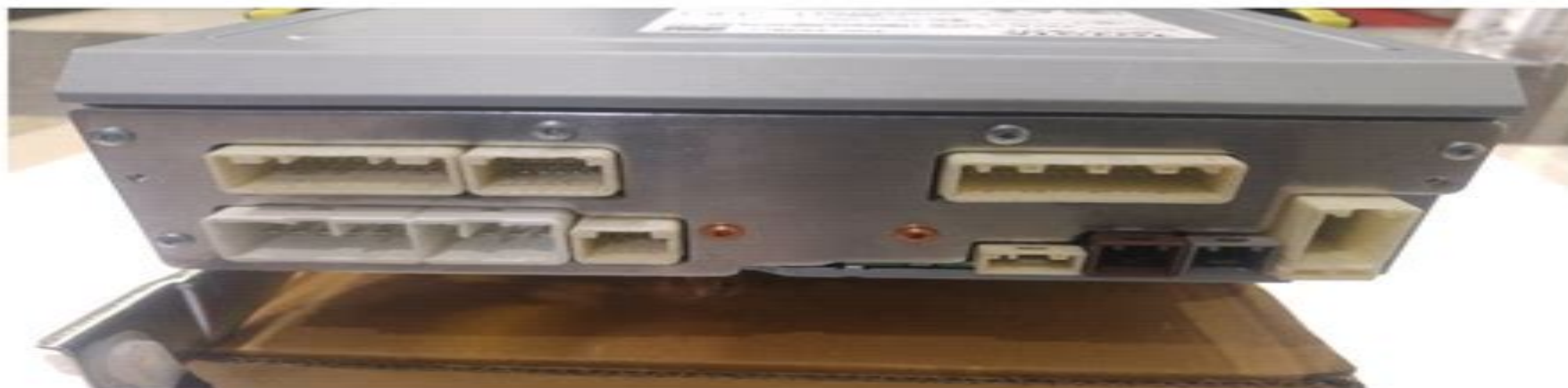
16 pin (10+6) Toyota Head Unit proprietary connector
