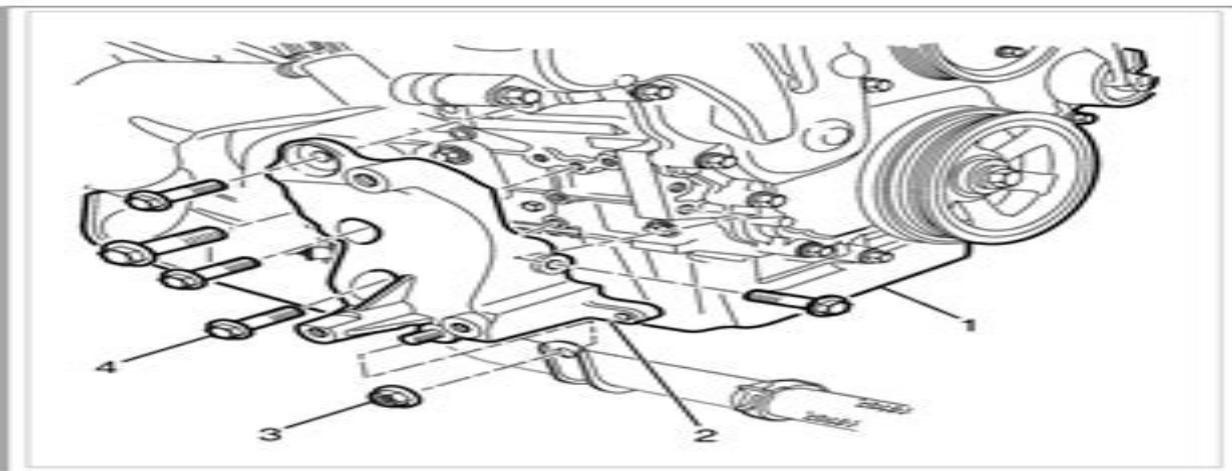
2. Remove the coolant inlet pipe to alternator mounting bracket retaining nut (3).
