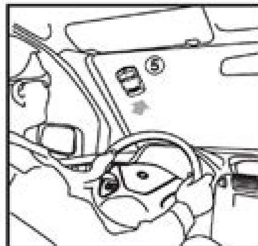
**WARNING:** Do not place or store the CarKit over the area of the automobiles safety airbag deployment, or it may cause serious injury when a safety airbag deploys.
