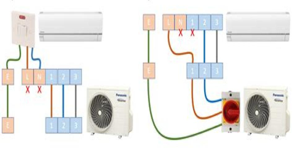
Applies to RE, TE, FE, FZ, TZ, Z, XZ models. Note where the LIVE wires to for each option
