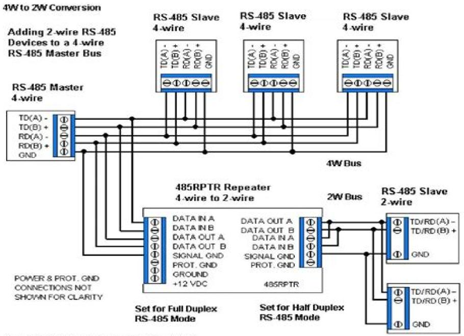
Note: 2W Master is not able to support 4W devices without data loss
