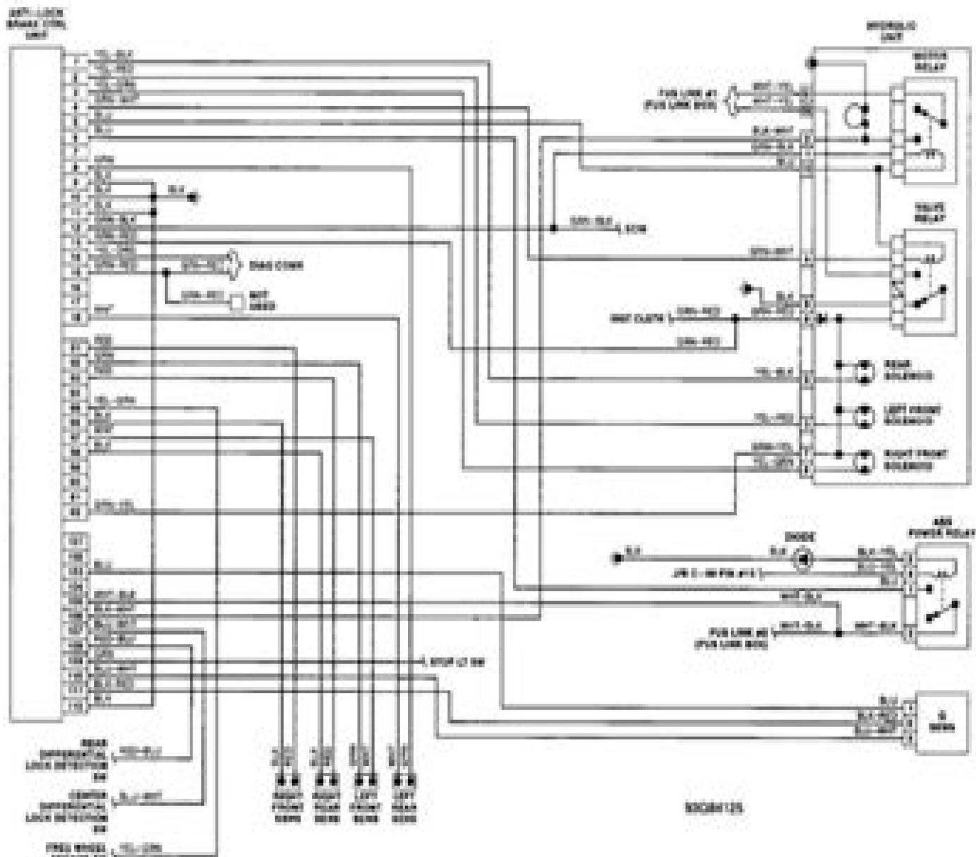
Fig. 20: Anti-Lock Brake System (ABS) Wiring Diagram
